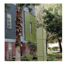
North 42 used HPL rainscreen panels to give a new look to the campus housing apartments. The Plus5 bracket system attached directly back into the existing wall. The complex also used the HPL panels to create signage around the apartment complex.
