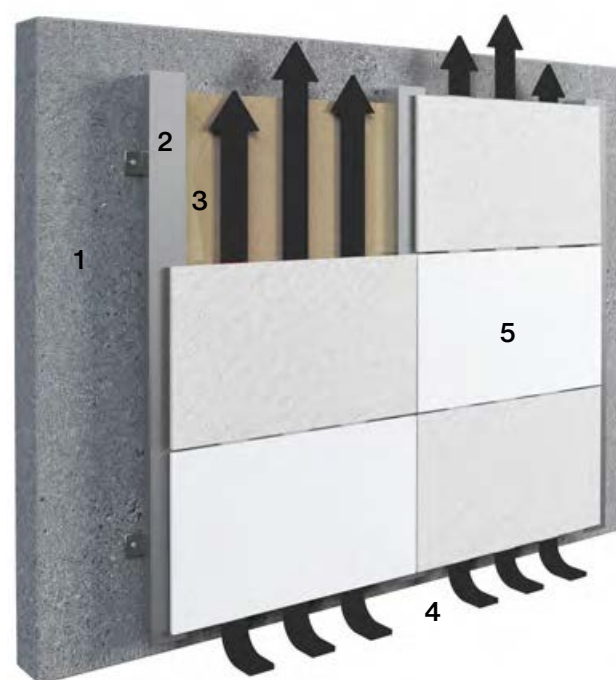
1 Supporting structure, 2 Substructure, 3 Thermal insulation, 4 Rear ventilation space, 5 Swisspearl fibre cement panels
